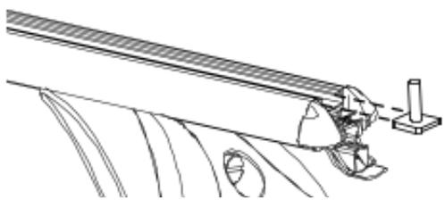
End cap can be opened to remove the rubber strip & insert T-Bolts for ease of adding accessories. You will need to cut the rubber strip to reinsert around the T-Bolts, and maintain the weatherproofing of the roof bars.
